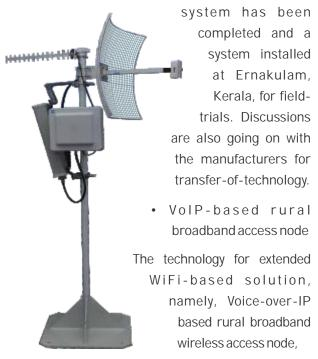
has been enhanced with capabilities of repeater-mode operation, and cognitive radio to facilitate dynamic frequency allocation for efficient utilization of radio spectrum. The technology provides affordable broadband and end-to-end VoIP services in rural areas and can also be used for backhauling requirements. Field-trial is planned for the technology and a site has been identified for the purpose.
