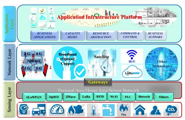
Figure 3: Typical Architecture of Smart City IoT Applications
