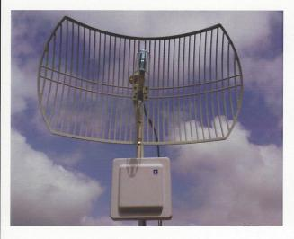
C-DOT long range Wi-Fi combines three unique benefits of three technologies into one, viz. long reach of optical fiber to take the high speed signal feed to 60 kms, spectrum sensing Wi-Fi solution to take the signal reliably beyond a great distance further; and Mesh technology which enables the signal to reach beyond Line of Sight as well as provides redundancy; ensuring reliable operations even in case of break of some links.
